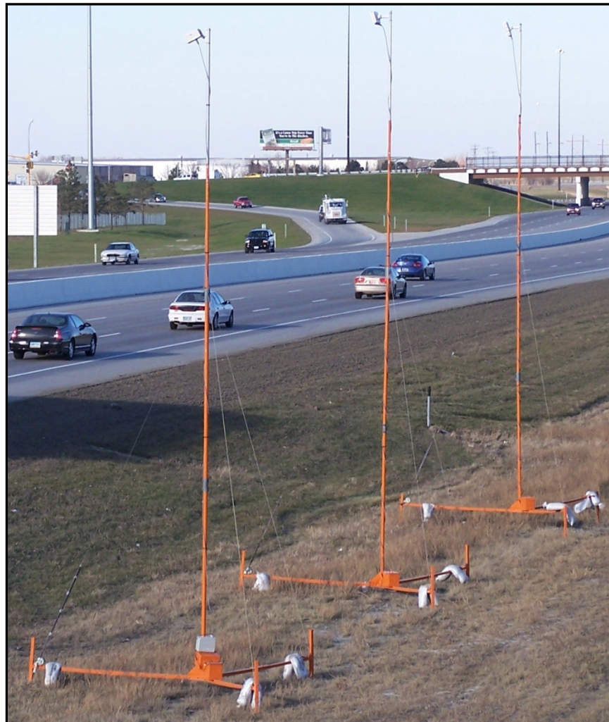
Figure 1. Radar Sensors on the Tripod Mounting System
