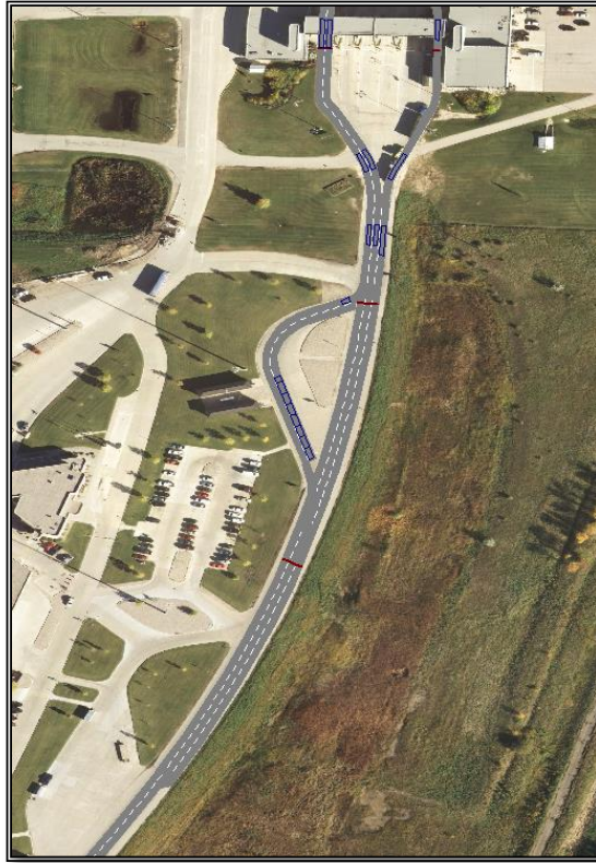
Figure 4 Alternative 2 Geometric and Traffic Control Changes
