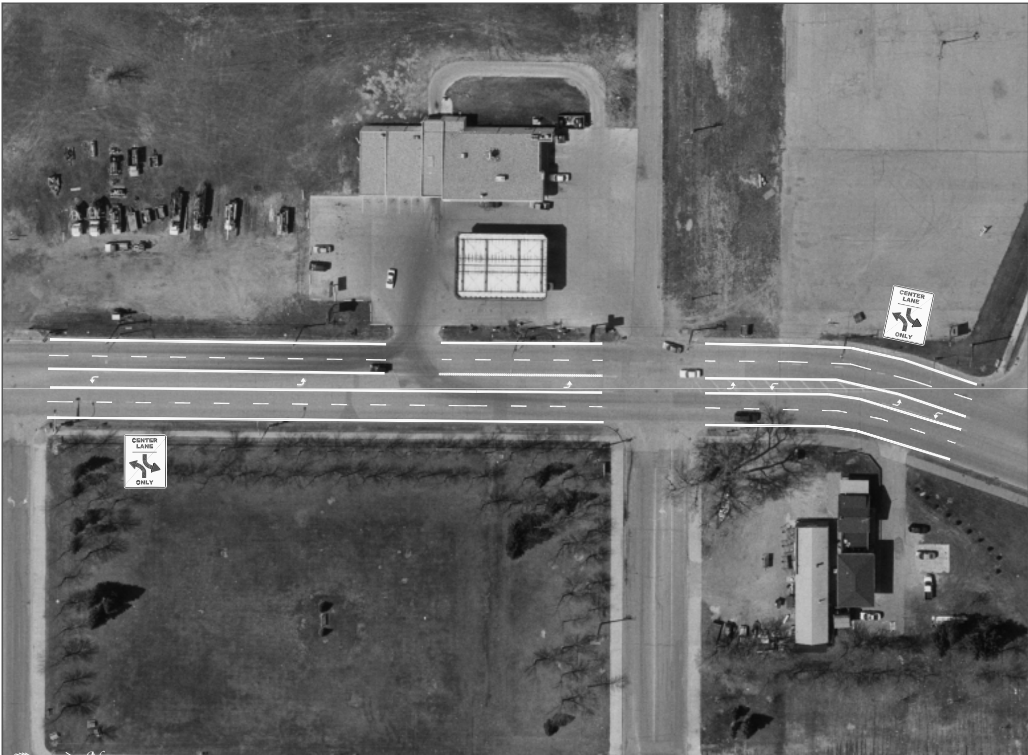
Figure 10. Two-Way Left Turn Lane Along 21st St. (1st Ave. S. - 4th Ave. S.)
